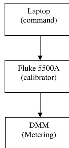
Figure 1. Block diagram of the calibration system
