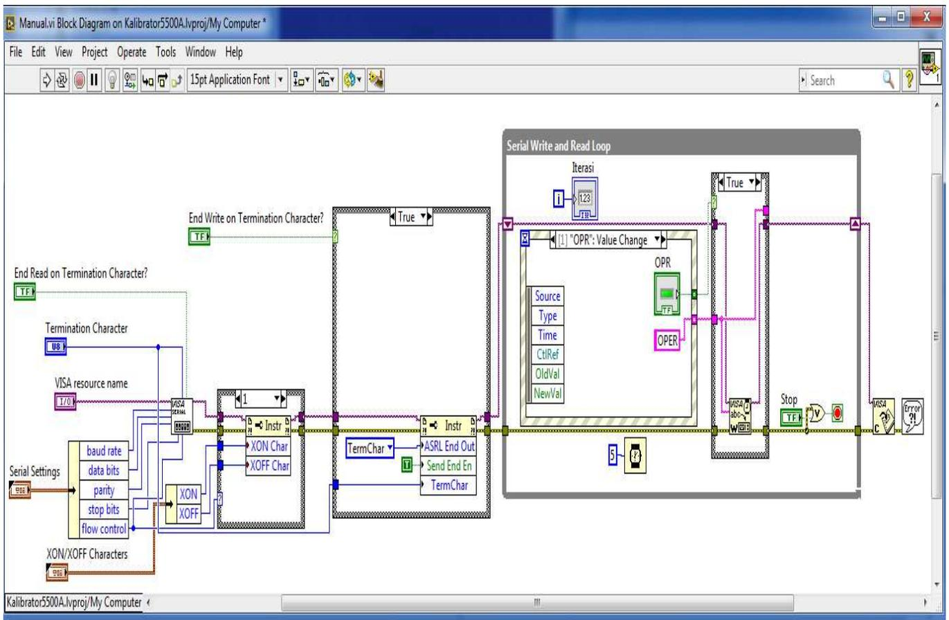
Figure 3. LabVIEW Block Diagram
